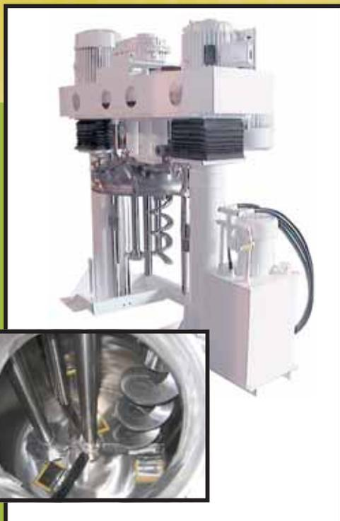
A unique blend of high speed, low speed and intermediate speed blades can vastly improve mixing times, product flow and homogenous results.
